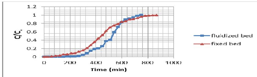
**Figure (8):** The Experimental Breakthrough Data for Adsorption of MB onto Commercial Activated Carbon at  $C_0=50$  mg/l,  $Q=12$  l/hr,  $L=0.1$ m,  $pH=5$ .
