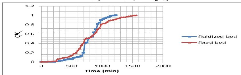
Figure (13): The Experimental Breakthrough Data for Adsorption of MB onto Commercial Activated Carbon at L=0.15 m, Q=12 l/hr, C<sub>0</sub>=50 mg/l, pH=5.
