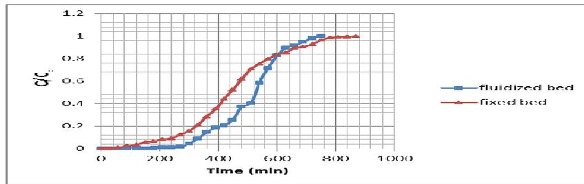
Figure (12): The Experimental Breakthrough Data for Adsorption of MB onto Commercial Activated Carbon at L=0.10 m, Q=12 l/hr, C<sub>0</sub>=50 mg/l, pH=5.
