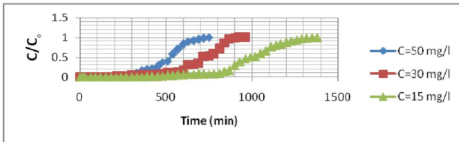
**Figure (5):** The Experimental Breakthrough Data for Adsorption of MB onto Commercial Activated Carbon at Different Initial Concentrations, Q=12 l/hr, L=0.1m, pH=5.
