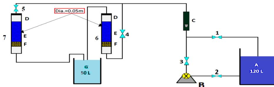
**Figure (1):** Schematic Representation of Experimental Equipments. (A) Feed Tank, (B) Pump, (C) Rotameter, (D) Perforated Plate in Fixed Bed and Stainless Sieve in Fluidized Bed, (E) Packed Bed Adsorbent, (F) Class Beads & Stainless Sieve, (G) Effluent Tank, (1,2,3,4&5) Valves, (6) Expanded Bed Adsorbent and (7) Packed Bed Adsorbent.
