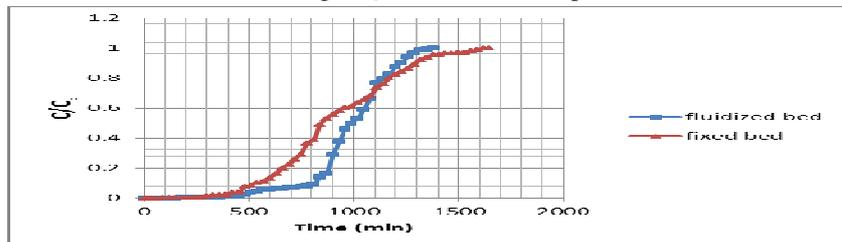
**Figure (10):** The Experimental Breakthrough Data for Adsorption of MB onto Commercial Activated Carbon at  $C_0=15$  mg/l,  $Q=12$  L/hr,  $L=0.1$ m,  $pH=5$ .
