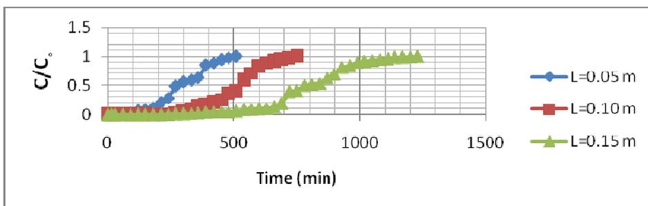
**Figure (6):** The Experimental Breakthrough Data for Adsorption of MB onto Commercial Activated Carbon at Different Bed Depths, Q=12 l/hr, C<sub>0</sub>=50 mg/l, pH=5.
