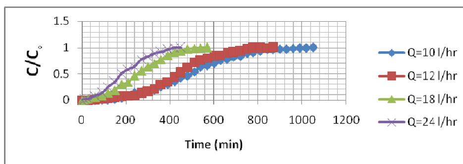
**Figure (4):** The Experimental Breakthrough Data for Adsorption of MB onto Commercial Activated Carbon at Different Flow Rates,  $L=0.1$  m,  $C_0=50$  mg/l,  $pH=5$ .
