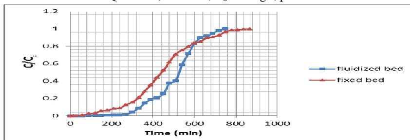
Figure (15): The Experimental Breakthrough Data for Adsorption of MB onto Commercial Activated Carbon at Q=12 l/hr, L=0.1 m, C<sub>0</sub>=50 mg/l, pH=5.
