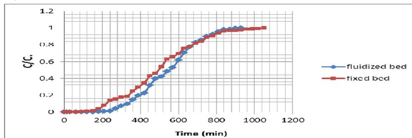
Figure (14): The Experimental Breakthrough Data for Adsorption of MB onto Commercial Activated Carbon at Q=10 l/hr, L=0.1 m, C<sub>0</sub>=50 mg/l, pH=5.
