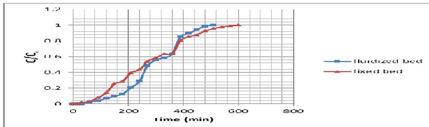
**Figure (11):** The Experimental Breakthrough Data for Adsorption of MB onto Commercial Activated Carbon at  $L=0.05$  m,  $Q=12$  l/hr,  $C_0=50$  mg/l,  $pH=5$ .
