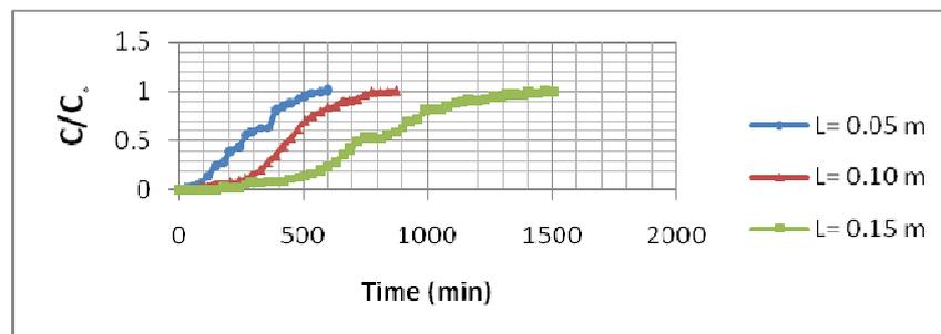
**Figure (3):** The Experimental Breakthrough Data for Adsorption of MB onto Commercial Activated Carbon at Different Bed Depths,  $Q=12$  l/hr,  $C_0=50$  mg/l,  $pH=5$ .
