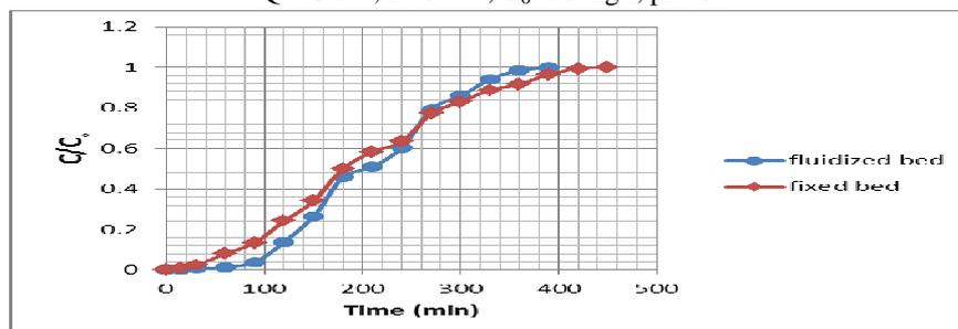
**Figure (17):** The Experimental Breakthrough Data for Adsorption of MB onto Commercial Activated Carbon at  $Q=24$  l/hr,  $L=0.1$  m,  $C_0=50$  mg/l,  $pH=5$ .
