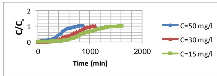
**Figure (2):** The Experimental Breakthrough Data for Adsorption of MB onto Commercial Activated Carbon at Different Initial Concentrations,  $Q=12$  l/hr,  $L=0.1$ m,  $pH=5$ .
