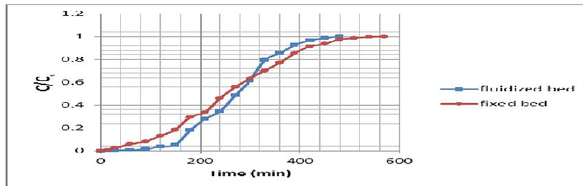
**Figure (16):** The Experimental Breakthrough Data for Adsorption of MB onto Commercial Activated Carbon at  $Q=18$  l/hr,  $L=0.1$  m,  $C_0=50$  mg/l,  $pH=5$ .
