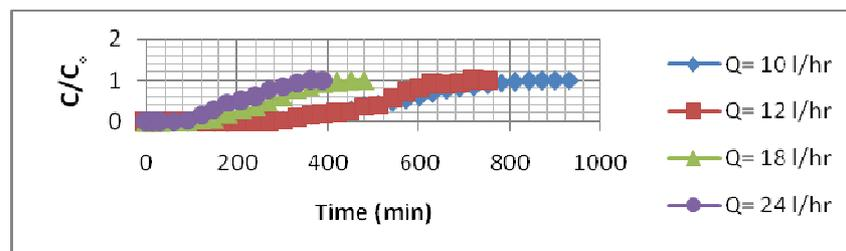
**Figure (7):** The Experimental Breakthrough Data for Adsorption of MB onto Commercial Activated Carbon at Different Flow Rates,  $L=0.1$  m,  $C_0=50$  mg/l,  $pH=5$ .
