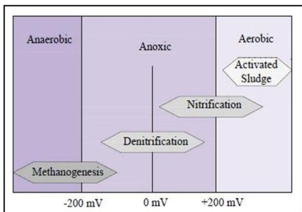
Figure 1: ORP ranges (mV) for typical wastewater processes [9].
