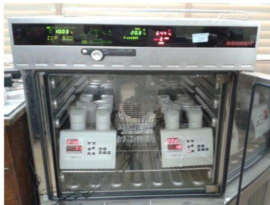
Figure 8: Lovibond BOD-system OxiDirect and its incubator
