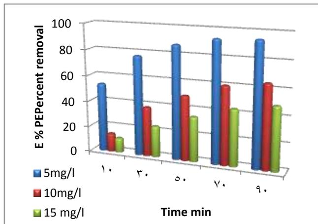
Fig.3: Effect of initial dye concentration on the removal of methylene dye removal
