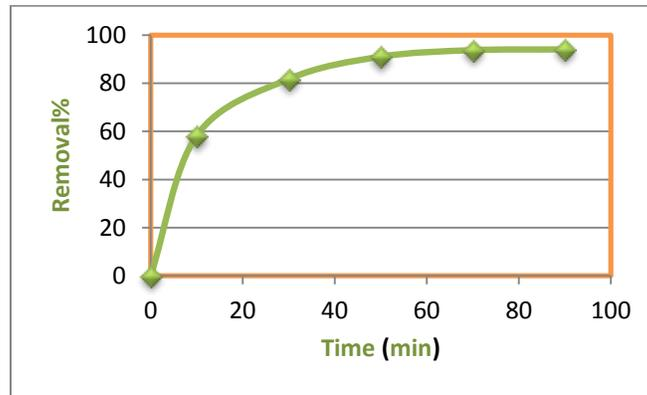
Fig.1: relation between contact time and removal efficiency
