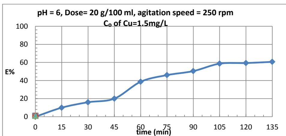
Fig.1. removal efficiency of  $\text{Cu}^{+2}$  on egg shell as a function of contact time
