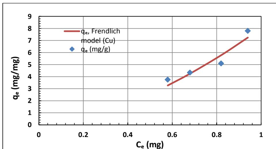
Fig. 6: Comparison of the experimental results with the  $q_e$  values obtained by Freundlich isotherm model for Cu<sup>+2</sup> sorbed by egg shell.
