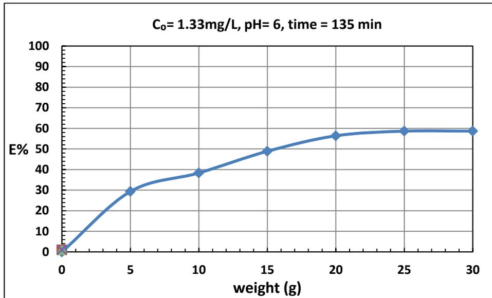
Fig. 3Effect of egg shell dosage on removal efficiencies of Cu<sup>+2</sup>.
