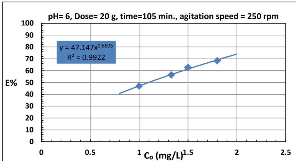
Fig 4. Effect of initial concentration on the removal efficiency of Cu+2 on egg shell
