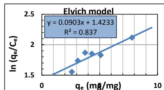
Fig.5 Linear isotherm models for sorption of Cu<sup>+2</sup> onto eggshell (Co=1.33 mg/l, pH=6, agitation speed=250 rpm, contact time=105 minute).
