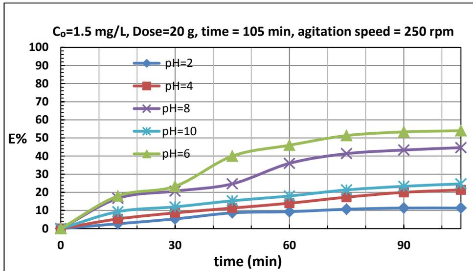
Fig. 2 removal efficiency of Cu<sup>+2</sup> with egg shell at different pH solution.
